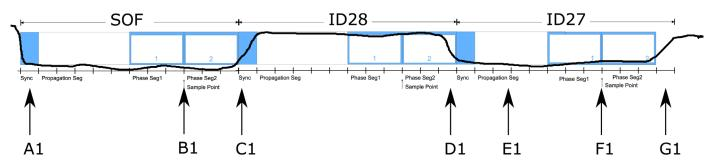
Figure 1: Alteration of phase shift due to oscillator tolerance by adjusting the number of time quanta (Source: Kvaser)
