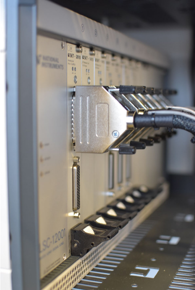
Figure 3: Modular system architecture using SLSC (Source: SET)
