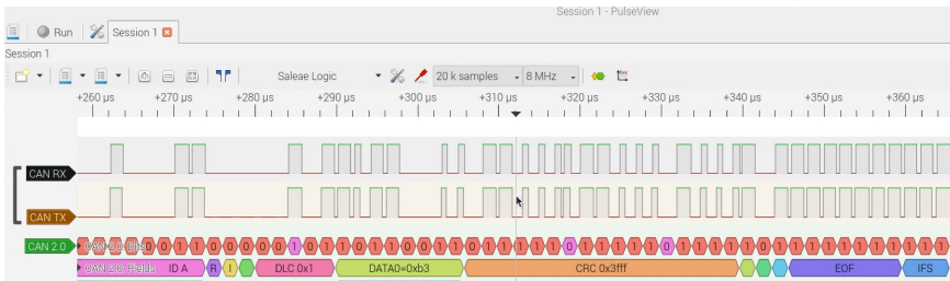
Figure 1: Logic analyzer trace of a Janus frame (Source: Canis Automotive Labs)
