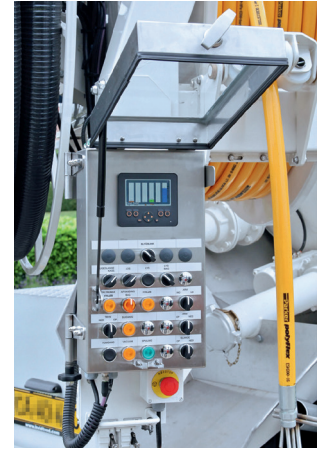
Figure 3: The Basicdisplay CR0451 indicates the most important parameters on the control panel (Source: ifm)
