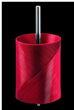
Figure 2: At the heart of the DC miniature and micro-motors is the patented, self-supporting, coreless rotor coil with skew-wound design, which rotates around a fixed magnet (Source: Faulhaber)
