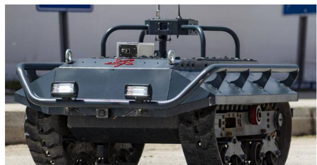
Figure 3: Havelsan's CAN-based unmanned ground vehicle (Source: CSS Electronics)
