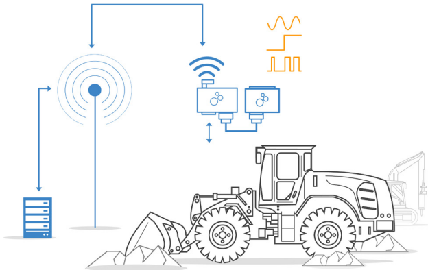
Figure 7: Add-on module for data acquisition and telematics (Source: CSS Electronics)
