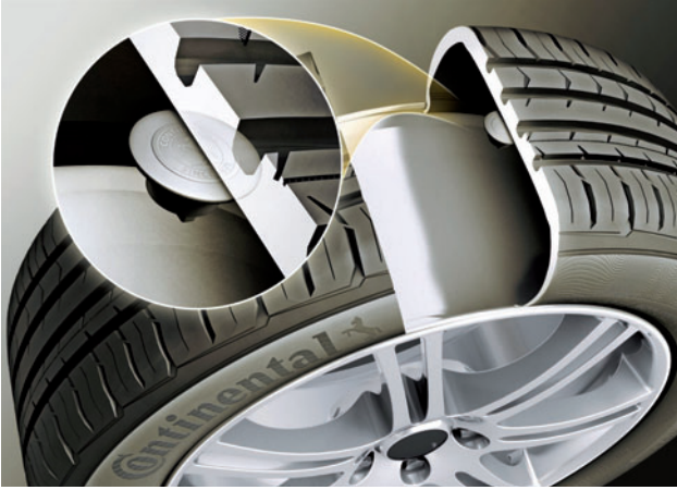
Figure 1: Being integrated directly into the inner liner of the tire means that the eTIS sensor offers data to the CAN-based receiver unit that can be forwarded to interested ECUs (Photo: Continental)
