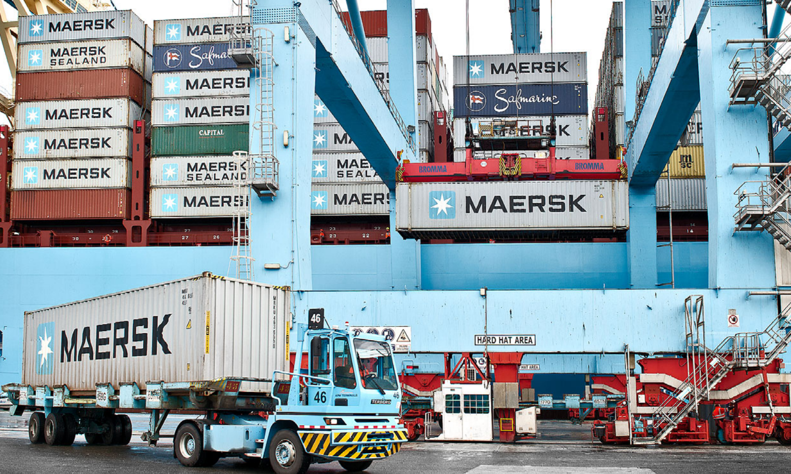
Figure 4: Bromma has delivered crane spreaders to 500 terminals in 90 nations, since more than 10 years they use embedded CANopen networks as well as an optional CANopen interface to communicate with the crane controller (Photo: Maersk)
