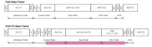
Figure 1: CAN frame layout (Photo: Goepel)
