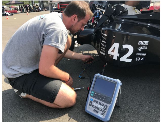
Figure 4: Niklas Waldstein measuring the engine control unit of the F17 to test ignition interruption (Source: FaSTDa Racing Team)
