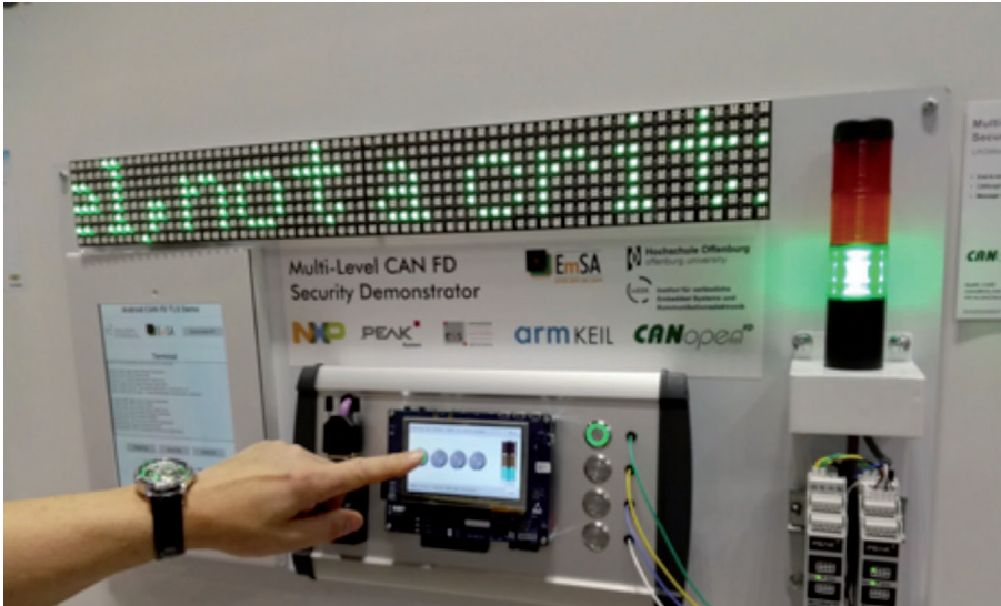
Figure 7: The CANopen multi-level security demonstrator by NXP (Source: Emsa)
