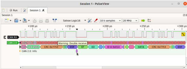
Figure 4: Warning about a double receive (Source: Canis Automotive Labs)
