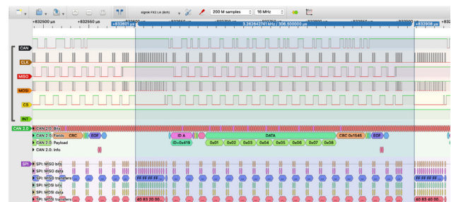
Figure 9: CAN traffic after driver optimization reducing the time between frames (Source: Ian Tabor)
