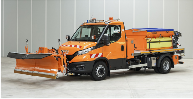
Figure 5: Iveco Daily with Kuepper Weisser winter equipment and Unsinn roll on/off system (Source: Iveco)
