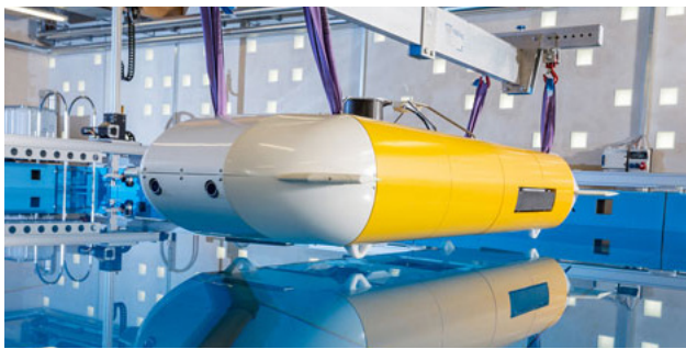
Figure 5: The 3,5-m-long AUV weighs less than 700 kg and provides a slim CAN architecture (Source: Fraunhofer IOSB-AST)
