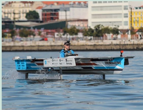
CAN-controlled hydrofoils allow the SR02 boat to get elevated over the water line, thus reducing the drag forces and the energy consumption (Source: Kvaser)
