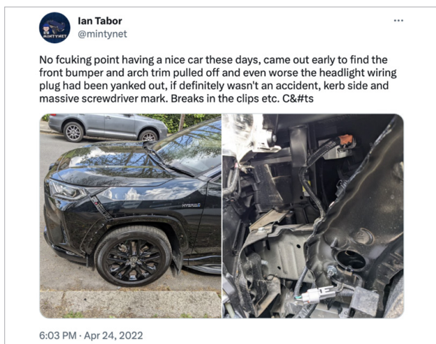
Figure 1: A tweet from Ian Tabor a few weeks before the car was stolen, showing how the ‘vandalism’ was actually an attempted CAN Injection attack (Source: Ian Tabor, Twitter)
