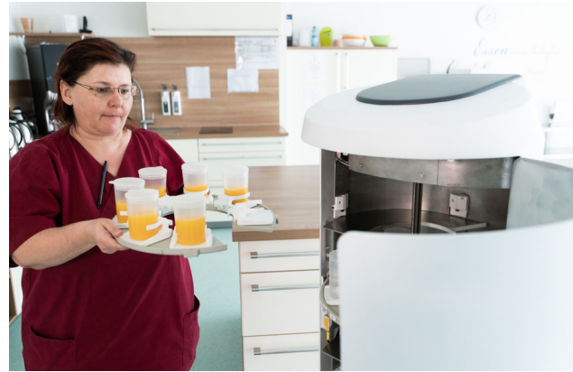
Figure 3: The service assistant can hold up to 28 cups or various snacks (Source: IPA Fraunhofer)
