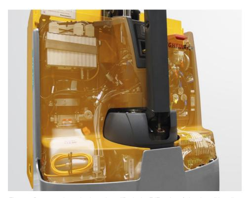
Figure 1: Data recorder and universal amplifier in the EJE series of electric walkie pallet trucks (Source: HBM/Jungheinrich)
