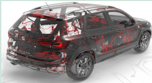
Figure 5: In some of today's Seat models there are more than 12 000 wiring combinations; this figure could increase in the future (Source: Seat)
