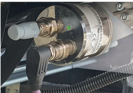
Figure 1: Horizontal drills from AT-Boretec use the WDGA CANopen encoder from Wachendorff for accurate drilling and automated reloading of the drill pipes (Source: Wachendorff)
