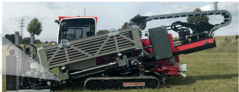
Figure 1: Horizontal drills from AT-Boretec use the WDGA CANopen encoder from Wachendorff for accurate drilling and automated reloading of the drill pipes (Source: Wachendorff)
