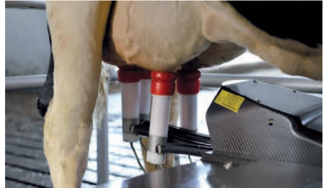
Figure 2: After going in the box the robotic arm moves under the cow, scans it with lasers to find the teats, and attaches four teat cups (Source: Lely)
