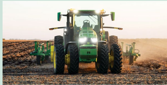
Figure: The 8R tractor uses cameras and artificial intelligence to navigate (Source: John Deere)
