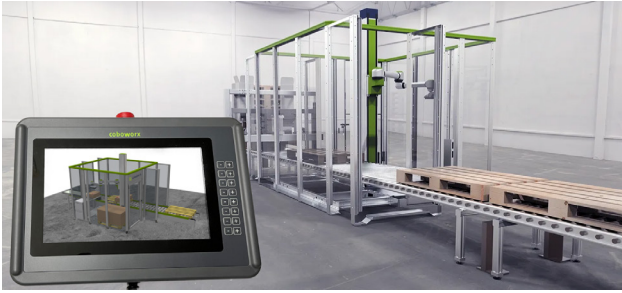
Figure 2: Coboworx pelletizing cell and panel with the digital twin of the plant (Source: Coboworx, Machineering)
