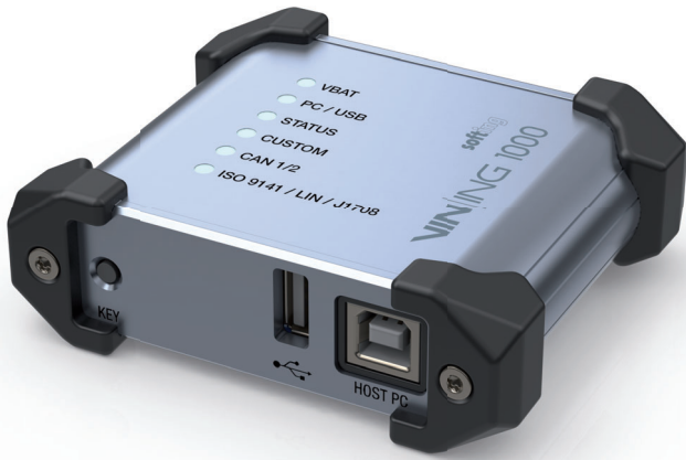
Figure 1: VIN-ING 1000 - Compact VCI for simple service diagnostics (Photo: Softing)
