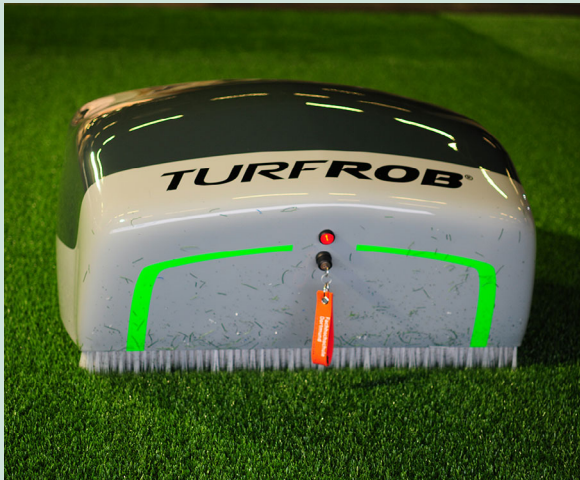
The Turfrob is equipped with three drives, which communicate with the host controller via CANopen (Photo: Dunkermotoren)
