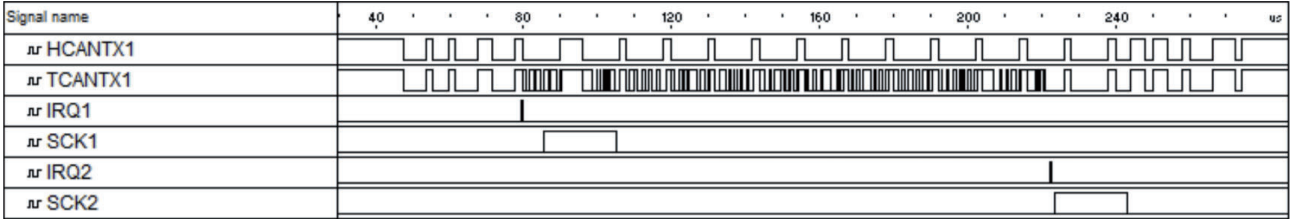
Figure 6: Logic analyzer trace of a received CAN-HG frame (Photo: Canis)
