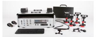
Figure 1: The VTK comprises several hardware components and the D-Lab software platform (Photo: Ergoneers)
