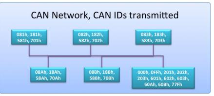
Figure 1: CAN-IDs used for transmissions (Source: Emsa)
