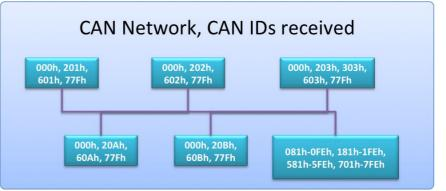
Figure 2: CAN-IDs of received data frames (Source: Emsa)
