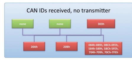
Figure 3: "Unprotected" CAN-IDs (Source: Emsa)
