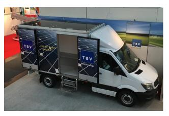
Figure 2: The refrigerated van from TBV uses integrated PV modules to support the refrigeration of the compartment (Source: TBV Kühlfahrzeuge)
