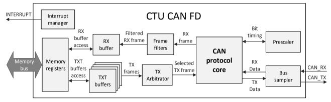
Figure 1: CTU CAN FD IP core structure (Source: CTU)
