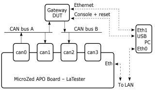
Figure 2: Testing setup for latency testing (Source: TCU)
