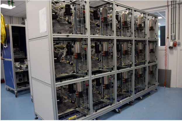
Figure 1: Re/genT uses measurement and control equipment to assess how a compressor and its electronic components can be further optimized (Source: Re/genT, Keller Meettechniek)
